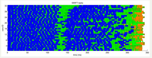
Each core has it's own task queue and uses work-stealing when empty.
