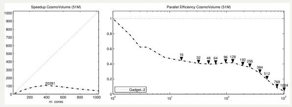
**51M particle EAGLE box** (z = 0.5) SPH-only simulation on the COSMA5 cluster.
